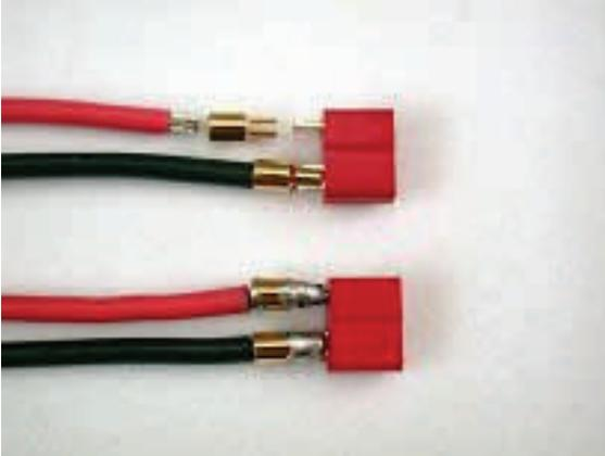
for the wire and two prongs that fit tightly over the blades on the Deans. They will accept up to 12 gauge wire and are so much easier. I like that they seem to give a higher level of mechanical integrity to the connection that will get pulled on. G-force hobbies usually
