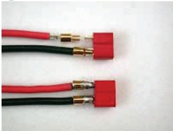
for the wire and two prongs that fit tightly over the blades on the Deans. They will accept up to 12 gauge wire and are so much easier. I like that they seem to give a higher level of mechanical integrity to the connection that will get pulled on. G-force hobbies usually
