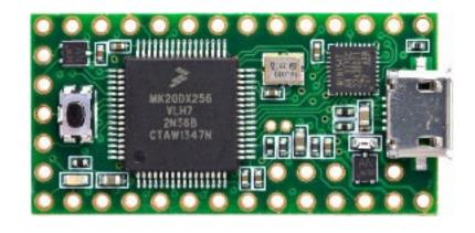
mini-USB), it has a much faster processor, more memory, 3 hardware serial ports, 21 analog input ports, 2 analog digital converters, an output digital to analog converter. 12 PWM pins, and it is 5 volt tolerant. Wow. Cost \$24 shipped. Oh well, I'll find a use for the Arduino mini some day. I ordered the Teensy. In the mean time I got GPS and S.Port code from every source I could find.
