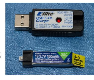
are around 7-8 minutes. Charging takes about 25 minutes, but batteries are cheap. I usually have 6 charged and ready to go at any given time. This is a big advantage over the Proto X, which has shorter flights and doesn't have swappable batteries. So, you fly for 3 minutes and charge for close to 30.
