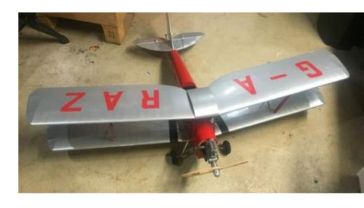
OS .40 four stroker on it and just needed a half ounce of lead on the tail to balance out. Took it to the field this past Saturday and couldn't get fuel into the tank. Hmmmm. Back to the bench for a re-check so no actual flight occurred yet. Dang it. Attached is the photo of my finished product.
