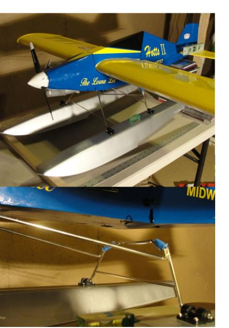
I am fitting my .25 size Midwest Hots II, to a set of .25 size E-flight Fiberglass floats. Currently, I am adjusting the height of the rear attachment point by cutting the pre-formed support, and then, solder it at the correct height.
